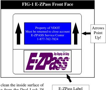
3. Having determined the mounting position in your vehicle, clean the inside surface of the windshield. Carefully remove the red protective backing from the Dual Lock <sup>TM</sup> mounting strips on the rear of the transponder. Firmly press the rear of the transponder against the glass. Maintain pressure for about 15 seconds to achieve a good bond.
