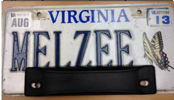
Fig- 2 Proper Mounting of Bumper E-Z Pass
