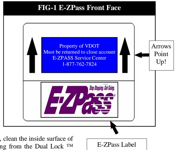
The transponder may be removed by lifting any one corner with sufficient pressure to separate the Dual Lock™ strips. Do not remove the Dual Lock™ strips and reuse them. Please obtain new strips from the Customer Service Center.
